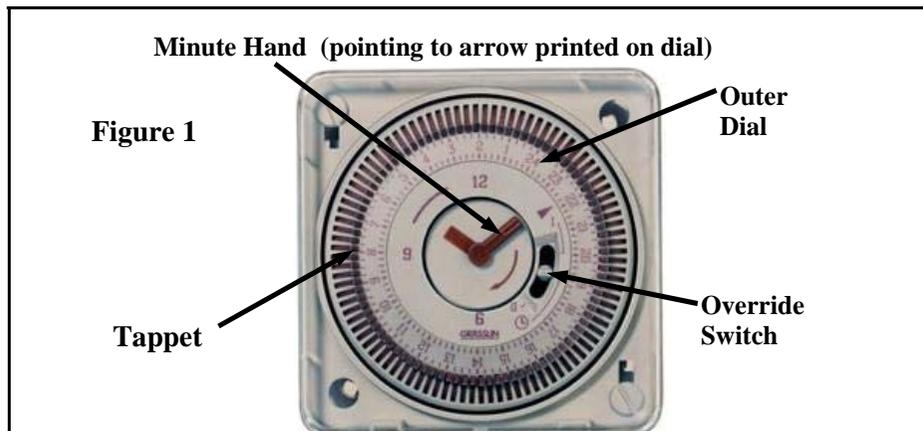
**Programming Switching Times** - Once the outer dial has been set to the current time you will need to position the appropriate tappets to your required on and off times. The factory set position of all tappets is in the off position, to change any tappets to the on position they must be switched away from the clock face. See Figure 2 Below.
