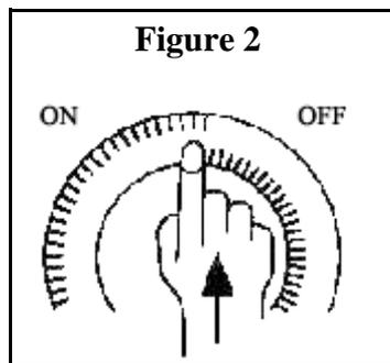
**Manual Override** - Your 24-hour timer is also fitted with a manual override switch that is built into the face of the dial illustrated in Figure 1 (top of page). This switch has 3 positions which are explained in the table on the following page.
