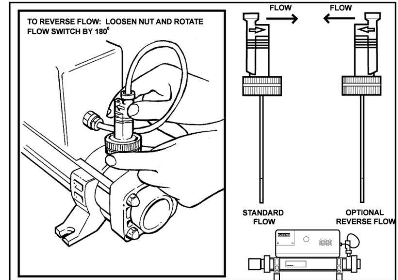
The flow rate of water entering the heater **must not** exceed 13,000-litres per hour (2,860 UK gallons per hour). A higher flow rate **will** require the installation of a bypass to prevent damage to the element(s).
